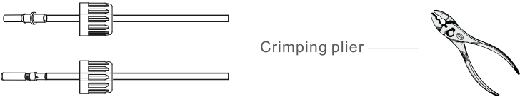
Pic 5.4 Crimp the contact pin to the wire
